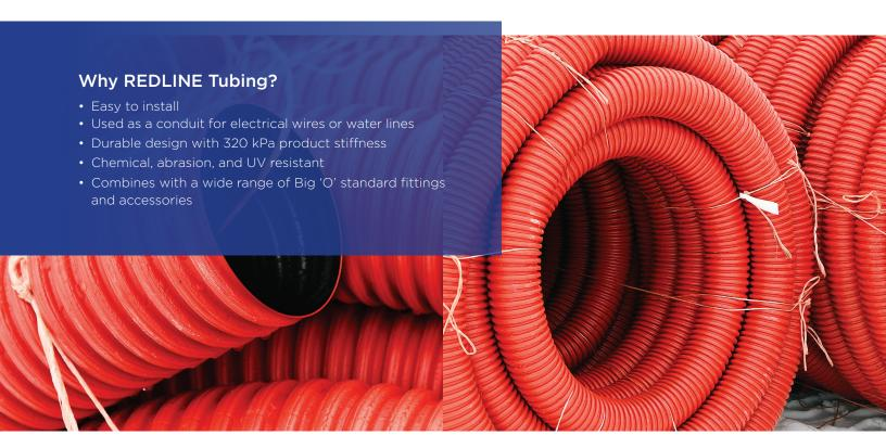
Big 'O' REDLINE corrugated tubing provides a safe and effective electrical conduit. The internal pull string simplifies installation, and its red colour ensures easy identification. REDLINE is available in 100 and 250 ft. lengths and conforms to BNQ 3624-115, but with a pipe stiffness of 320kPa.
