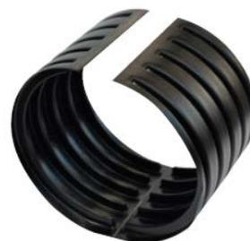
For damage greater than the width of a single corrugation, cut out the damaged area making cuts in the center of the corrugation valley. Cut the replacement pipe section to the desired length, trimming any
