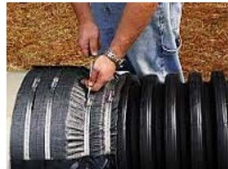
**FIGURE 2:** Dissimilar pipe coupler with rubberized sealing mastic and steel compression bands (*ref. Mar Mac*).
