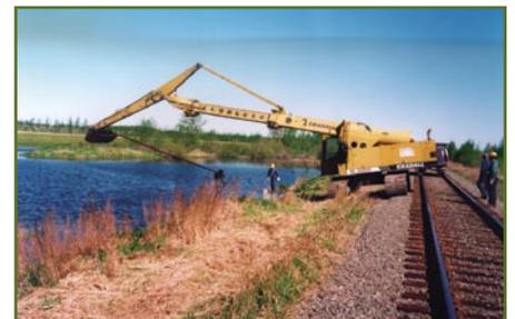
GRADALL WITH 30' SUPERBOOM EASILY CLEANS OUT PLUGGED CULVERTS.
